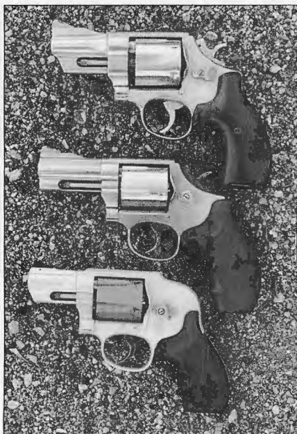
A trio of Smith & Wesson .44 Specials (from top to bottom): N-frame stainless steel M624 with 3-inch barrel, round butt and Skeeter Skelton style grip panels; L-frame stainless steel M696, also with 3-inch barrel and new AirLite Ti with 2.5-inch barrel.
